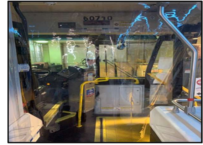
Driver / General Public Separation Barrier
